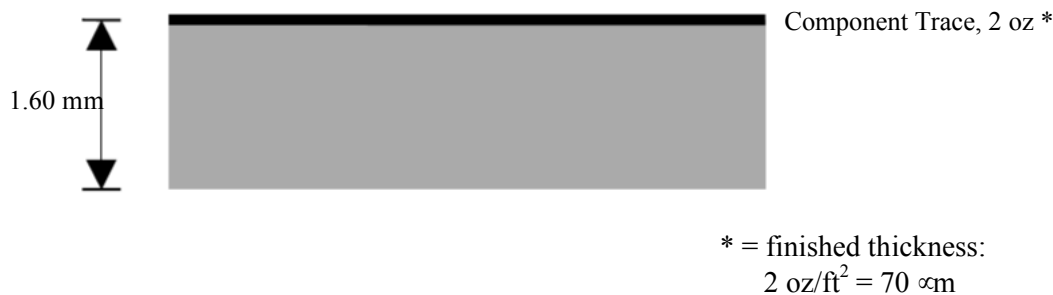
Figure 1a — Cross section of 1s PCB showing trace and dielectric thicknesses in package placement and trace fan-out regions
