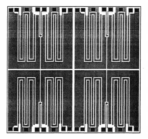
Figure 3. Multiple unit test chip layout (not to scale).
