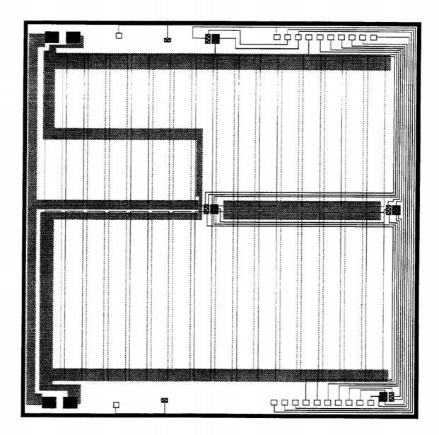
Figure 2. Single unit test chip layout (not to scale).
